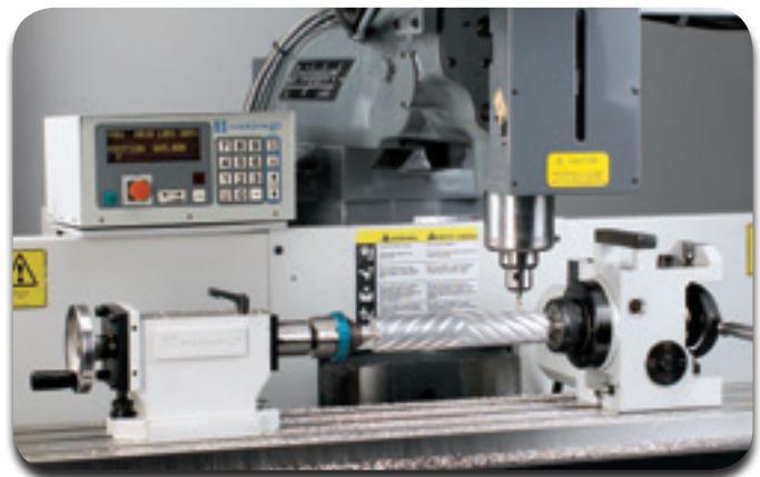
Spiral milling application on a Bridgeport knee mill using a 5C 2 indexer and manual tailstock.
